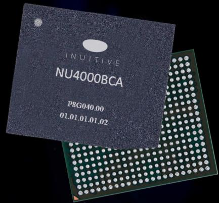
NU4000 is a superior multi core vision processor that supports 3D Imaging, Deep Learning and Computer Vision processing for Augmented Reality and Virtual Reality, Drones, Robots, and many other applications. This new generation processor enables high quality depth sensing, SLAM on-chip, Computer Vision and Deep Learning (CNN) capabilities; all in affordable form factor and minimized power consumption, leading the way for smarter user experiences.
